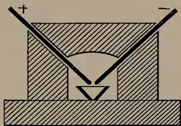
FIG. 128. An arc furnace
